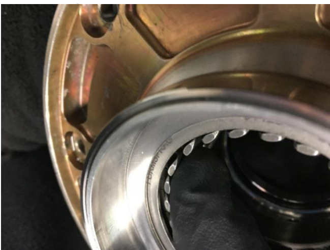
Sprags that mate direct to the smooth surface of the drive shaft
